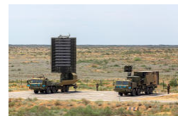
RLM-D and KU-RLK control cabin. Ministry of Defence of the Russian Federation, CC BY 4.0
